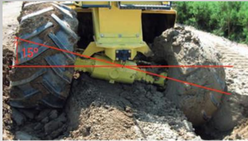
Non-spin oscillating axle \pm 15^\circ .
